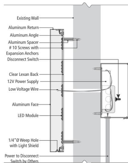
This sign is intended to be installed in accordance with the requirements of article 600 of the national electrical code and/or other applicable local codes. This includes proper grounding and bonding of the sign. The location of the disconnect switch after installation shall comply with Article 600.6(A)(1) of the National Electrical Code. All signs fabricated as per 2008 N.E.C. Standards.
