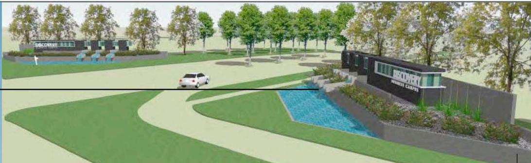
Smooth finish masonry or board form concrete or with anti-graffiti coating (by General Contractor). Sign company to coordinate footing with General Contractor. For bid purposes assume that general contractor will provide all masonry and/or concrete work including footing (design of footing by sign company). Sign to j-bolted to footer provided by GC.
