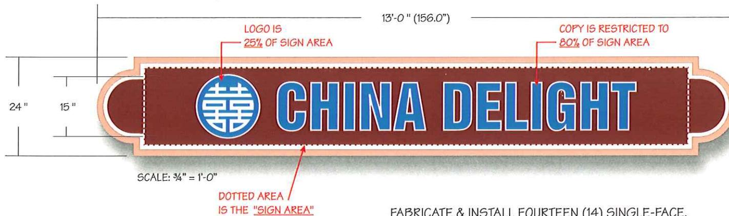
**FABRICATE & INSTALL FOURTEEN (14) SINGLE-FACE, ILLUMINATED, CEILING-MOUNTED CABINET SIGNS**
