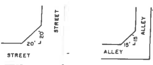
TYPICAL CUTOFF DETAIL
